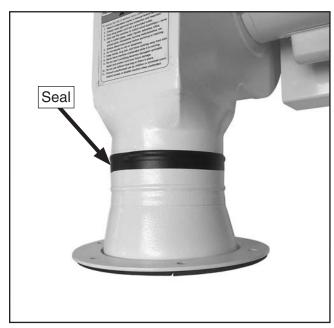
**Figure 4.** Electrical tape wrapped around seam between collection flange and outlet.
